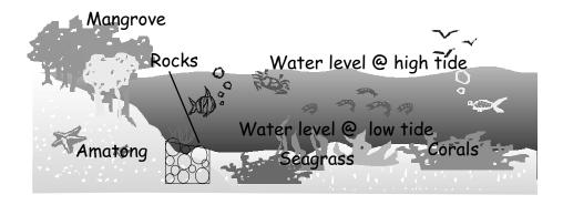
The Amatong can range in size from 2 to 4 meters in diameter or 2m x 4m in area and 0.5-1.5 meters deep. It may be circular, rectangular, or funnel-shaped. The distance between two amatong should be at least 50 meters. Harvesting is done after every 3-5 months by installing a net around the boulders and then removing the boulders one after another and piling them outside the Amatong. From 10 to 20 kg of the following fishes harvested from each amatong:
